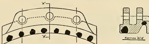
Side view and section of "FERALUN" BRAKE-SHOE showing where the Abrasive is placed
